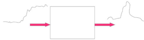
Fig. 4. The figure indicates that the filter's responsiveness should be greater at the edge location ( x=0 ) compared to its response at areas affected by noise, emphasizing the importance of achieving heightened sensitivity to genuine edge features while mitigating the influence of extraneous noise.
